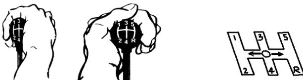
**1ST GEAR** is used for moving off, manoeuvring and for creeping slowly in traffic and at junctions.
