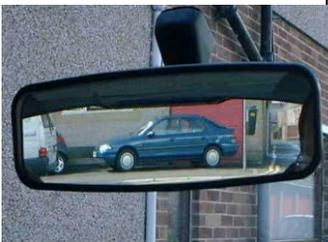
**MIRRORS** -You should be able to see clearly in the mirror with minimum head movement. When adjusting, hold the mirror keeping your fingers off the glass. Adjust the door mirrors so that the side of the car is just visible in order to reduce any 'blind spots'. The interior mirror is made of flat glass which gives you a true image of objects; the door mirrors are made of convex glass giving you a wider view but makes the object look smaller and further than it is.
